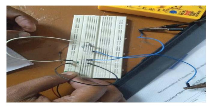
All the electronics experiments were made on the breadboard, allowing for easy construction and testing of circuits without the need for soldering. The breadboard provided a flexible and reusable platform for experimenting with various components, such as resistors, capacitors, transistors, and integrated circuits, enabling quick modifications and adjustments during the testing process.
