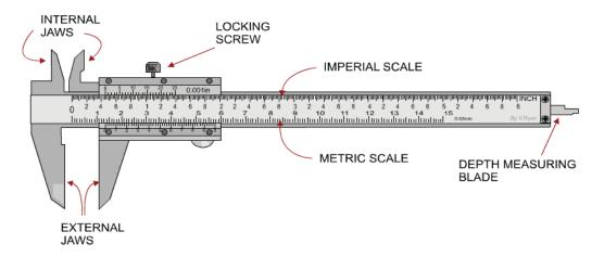
(iii) Measure the internal diameter and depth of a hollow cylindrical object: For measuring hollow objects like beakers, tumblers, or calorimeters, Vernier callipers help in determining the inner diameter and the depth (height). The volume of the hollow object is calculated using the formula for the volume of a cylinder, considering the inner dimensions.
