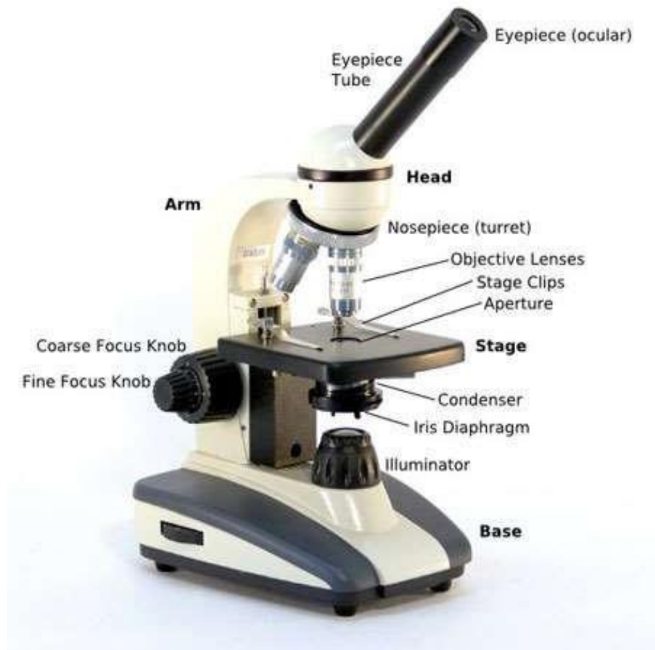
FIGURE: Showing Different Parts of Compound Microscope
