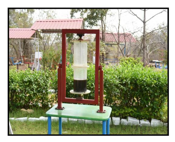
The rotating fluid subjected to centrifugal force creating funnel shaped formation like tornado. In this model the rotating fluid subjected to centrifugal force creating funnel shaped formation like tornado. A suitable modification was done to this model. Instead of water the tube has been filled with oil. As water evaporated so we have filled the tube with oil.
