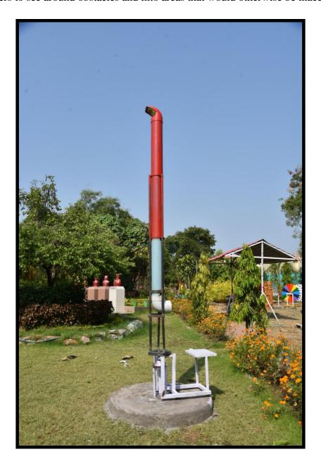
The Periscope Model comprises a series of mirrors or prisms arranged in a specific configuration to redirect light. A typical periscope consists of two parallel tubes, with mirrors placed at 45-degree angles at the top and bottom ends. This arrangement allows light to enter through the top mirror, reflect off the bottom mirror, and exit through the eyepiece, providing an observer with an elevated view of their surroundings.
