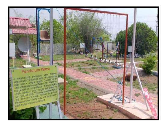
**Designing:** 13 independent pendulums have been fixed to a stable frame. Each pendulum has a different suspension length, and thus a different oscillation frequency. The lengths of the pendulum are adjusted in such a manner that if the longest pendulum executes L
